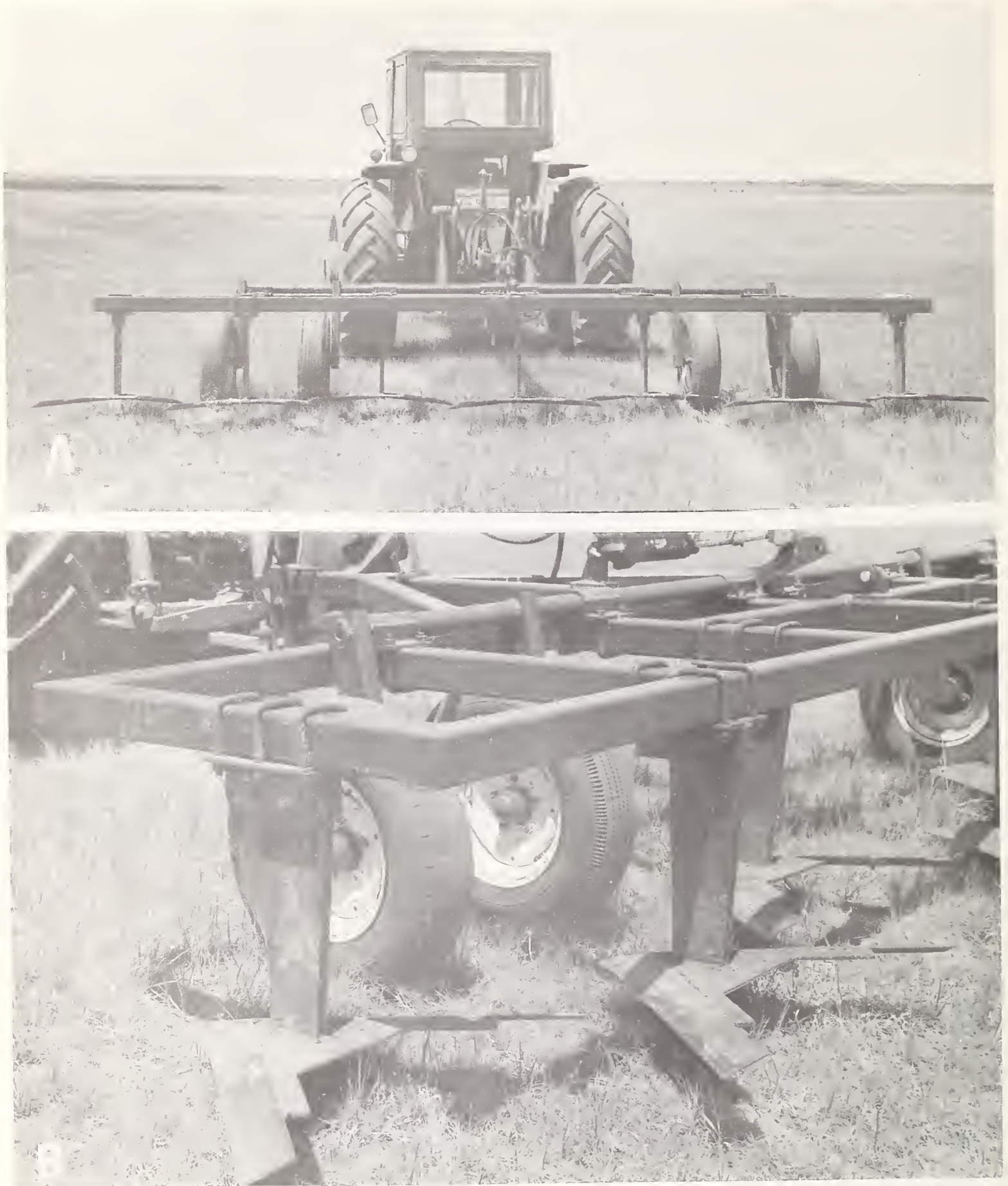
FIGURE 4.—A, Rear view of commercial stubble-mulch sweep plow used at the experiment station in 1969. The plow has seven, 36-inch sweeps and a total cut of 19 feet. B, Closeup view, showing simple, sturdy box frame and shank-and-sweep assembly.
